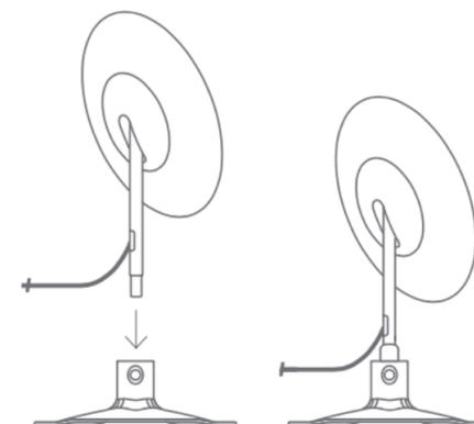
9. Place the mast of the Starlink into the hole at the center of the mount.
