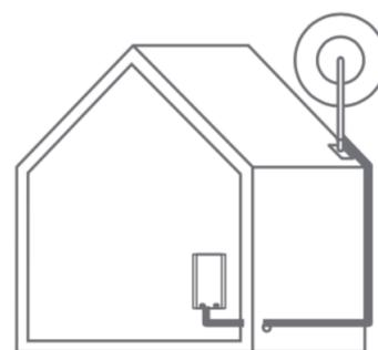
10. Unravel your connected cable coil. Route the loose end into your home and connect to the power supply.
