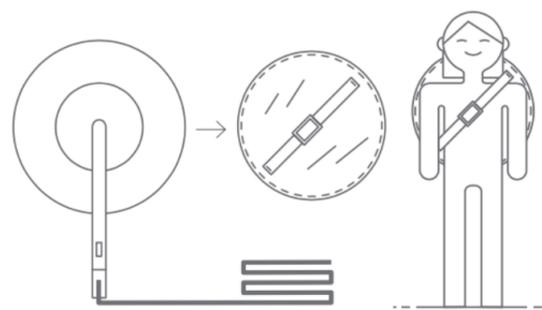
8. Place the Starlink and cable into the carrying bag and carry to the install location. Do not set the Starlink directly onto roof.
