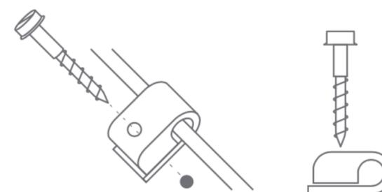
11. Use wall clips to fasten the cable to the wall along your route. Avoid puncturing cable and sharp bends, and follow horizontal/vertical lines.
